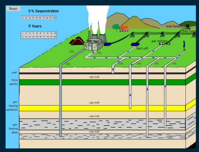
Layers shown: Coal, brine aquifer, gas bearing sandstone, gas bearing shale
